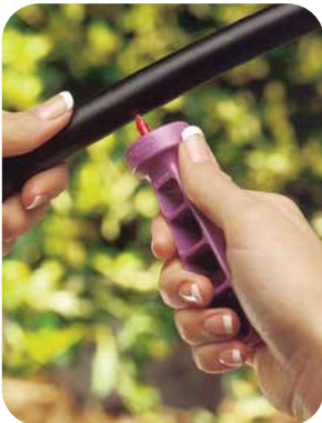
Use the Xeriman tool to quickly insert barbed fittings
